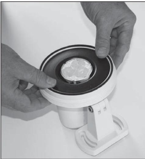
It is necessary to place the gasket exactly into its seat as shown in the picture. Then screw on gently the frame and tighten it by the key 4068469.
